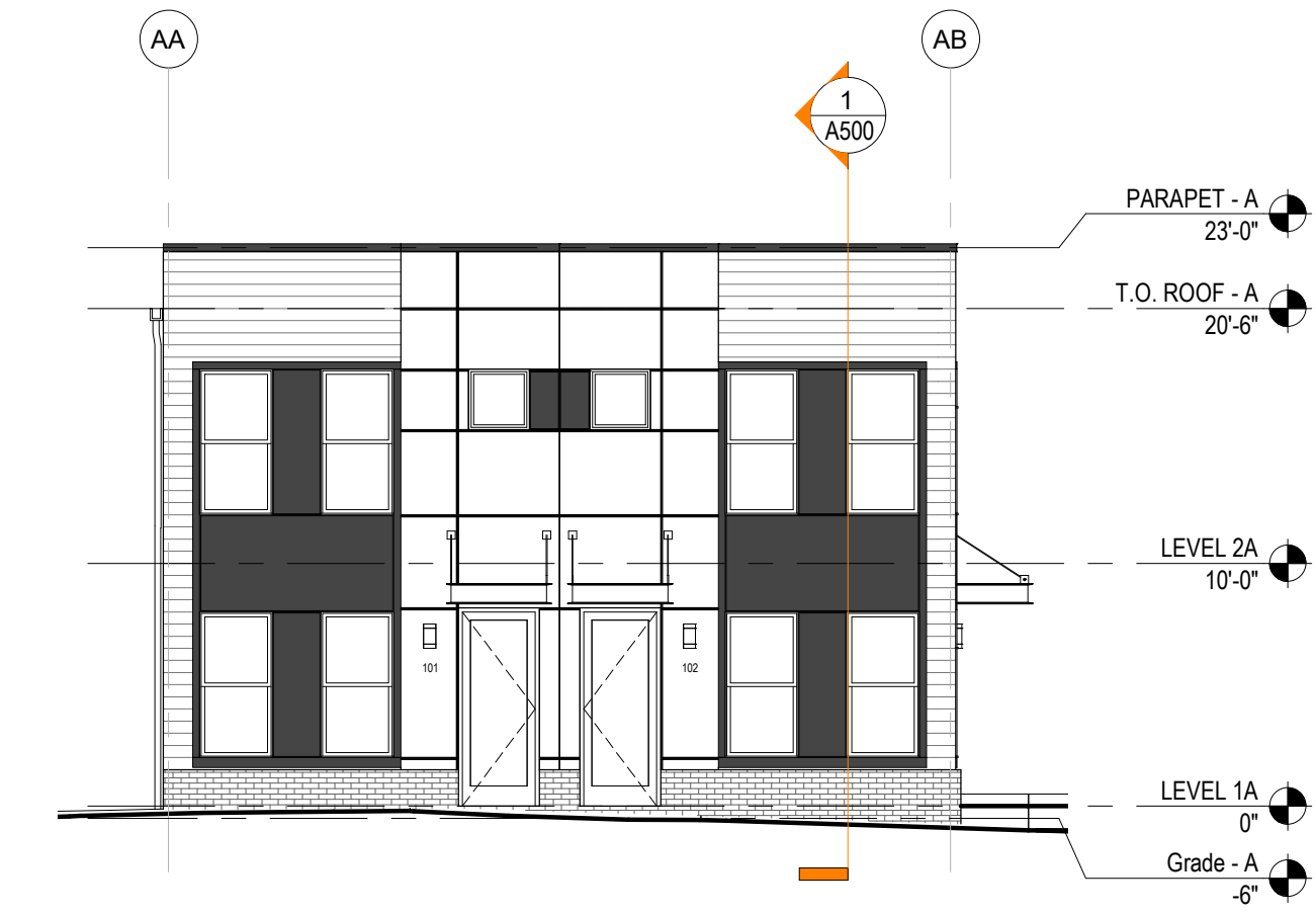
BUILDING A - SOUTH ELEVATION 3 1/8" = 1'-0" A400 A201-A
